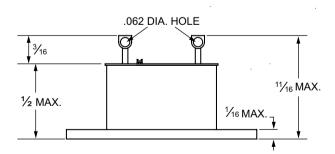
Direct replacement for Fenwal Series 32410/32411. The Fenwal Company discontinued this popular surface sensing series in 1987. The Warren G-V Series VE Thermostat mounts on the same 1.00" centerline as direct replacement, meeting all electrical and thermal requirements of the former unit.
