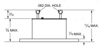
Direct replacement for Fenwal Series 32410/32411. The Fenwal Company discontinued this popular surface sensing series in 1987. The Warren G-V Series VE Thermostat mounts on the same 1.00" centerline as direct replacement, meeting all electrical and thermal requirements of the former unit.
